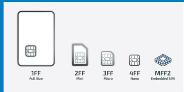
**EUICC (Embedded Universal Integrated Circuit Card):** A software standard that allows a single chip to host multiple SIM profiles. It also makes it possible to add, remove and manage these profiles over the air via a method called Remote SIM Provisioning (RSP). Usage of eUICC is not confined to Embedded SIM. It can be deployed with other SIM form factors, too. In short, with an eUICC, you can switch between carriers without the hassle of swapping SIM cards.
